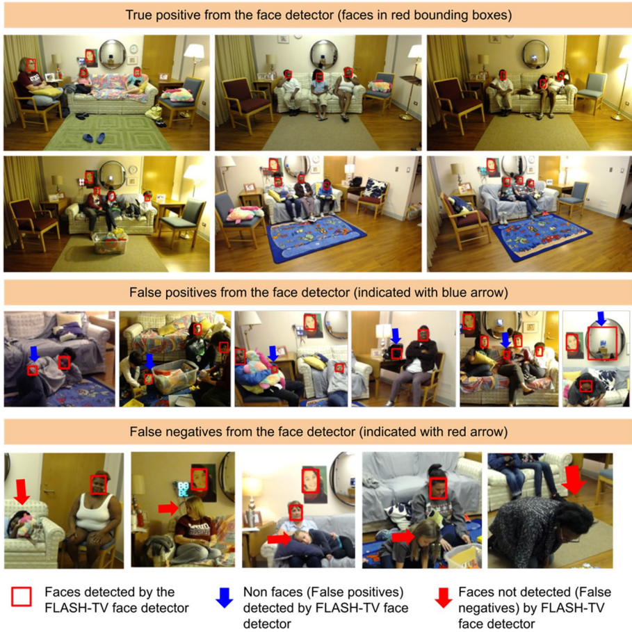
Fig. 7 FLASH-TV face detection results. Our detector is robust to various poses, low-lighting and low resolution
